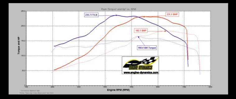
With kit fitted and mapped on our dyno the engine is now producing 231 BHP and a torque curve to match, the customers reaction initially was simply "WOW!" after the drive home.
